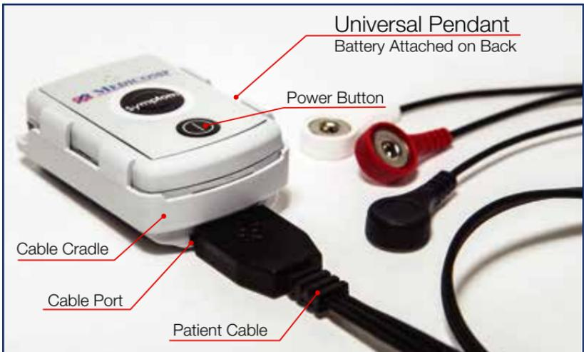
Clip the provided lanyard accessory onto the loop at the top of the Cable Cradle to wear it around your neck. Alternatively, you may carry it in your pocket but be careful that the Patient Cable remains firmly connected.
