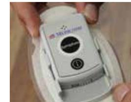
Insert the assembled Pendant into the cradle on the Electrode Patch. You should hear a click indicating the Pendant is securely inserted.
