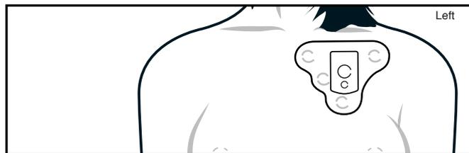
Press the Electrode Patch firmly on your skin in the proper position the left side of your chest. See illustration. Be careful not to press the buttons of the Pendant itself.
